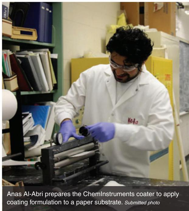
Anas Al-Abri prepares the ChemInstruments coater to apply coating formulation to a paper substrate. Submitted photo
